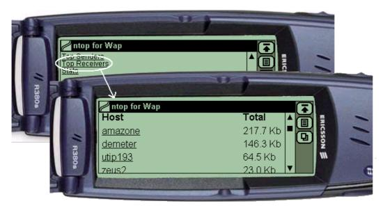
Figure 6 - ntop's WAP plug-in - accessing 'top receivers' from a WAP device
