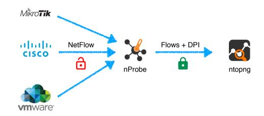
nprobe -3 <collector port> -i none -n none -zmq "tcp://\*:1234" --zmq-encryption-key <pub key>
