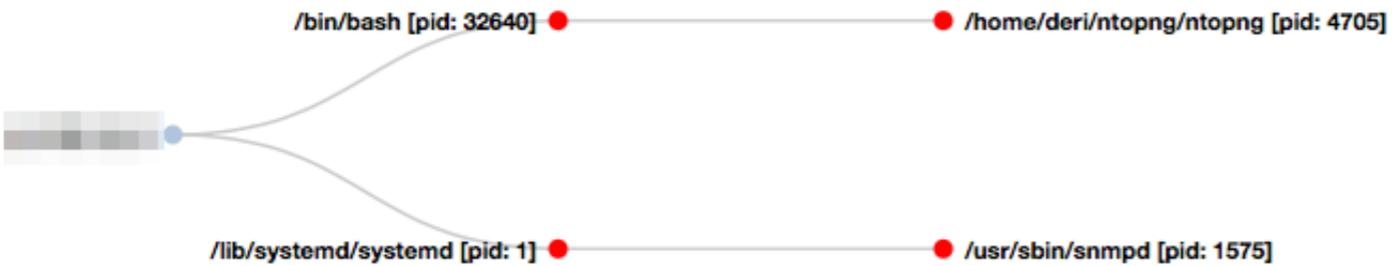
The diagram illustrates the process hierarchy. A blue host node at the bottom left connects to two red process nodes: '/bin/bash [pid: 32640]' and '/lib/systemd/systemd [pid: 1]'. These two processes then connect to another red process node: '/home/deri/ntopng/ntopng [pid: 4705]'. A legend indicates that blue dots represent hosts and red dots represent processes.
